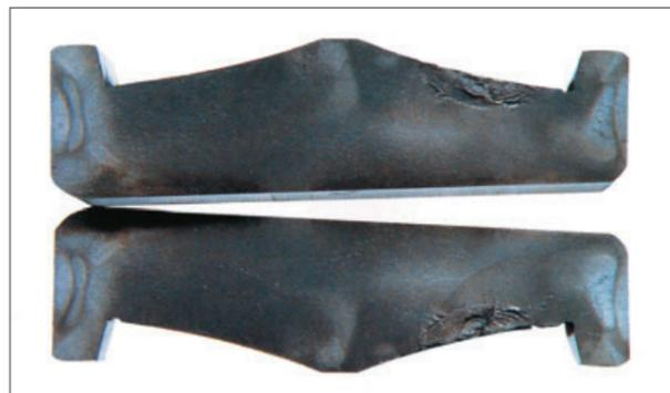
Part: Cross section of a fractured inner ring in a spherical roller bearing
