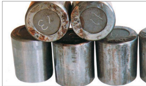
Part: Tapered rollers of a double-row tapered roller bearing
