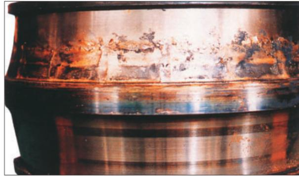
Part: Inner ring of a spherical roller bearing
