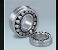
HPS series bearings are double-row self-aligning spherical roller bearings capable of carrying heavy radial loads with moderate axial loads in either direction. The spherical profile of the rollers, the inner ring raceway, and the outer ring raceway, enable a self-aligning function that allows full capacity loading. The HPS series offers high performance standard-size bearings with longer operating life and higher limiting speeds than conventional bearings.
