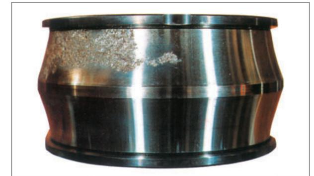
Part: Inner ring of a spherical roller bearing
