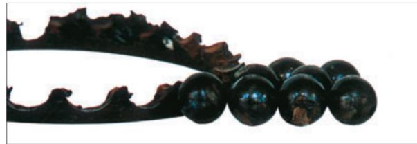
Part: Balls and cage of an angular contact ball bearing
