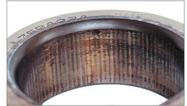
Part: Inner ring of an angular contact ball bearing
