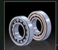
EM and EW series bearings are cylindrical roller bearings capable of carrying particularly large radial loads and are suitable for high-speed applications. The EW series features a pressed steel cage and the EM series features a one-piece machined brass cage. Both cages offer high-load capacity for standard-size bearings, in addition to excellent functionality and longer operating life.
