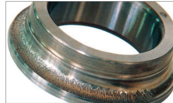
Part: Inner ring of an angular contact ball bearing
