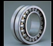
CA series bearings are double-row self-aligning spherical roller bearings with a machined brass cage that have a high load capacity, superior durability, and are resistant to wear. The CA series are especially suitable for applications that operate under heavy or shock load conditions.
