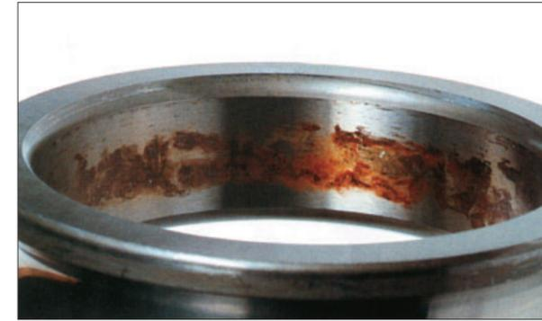
Part: Inner ring of a deep groove ball bearing
